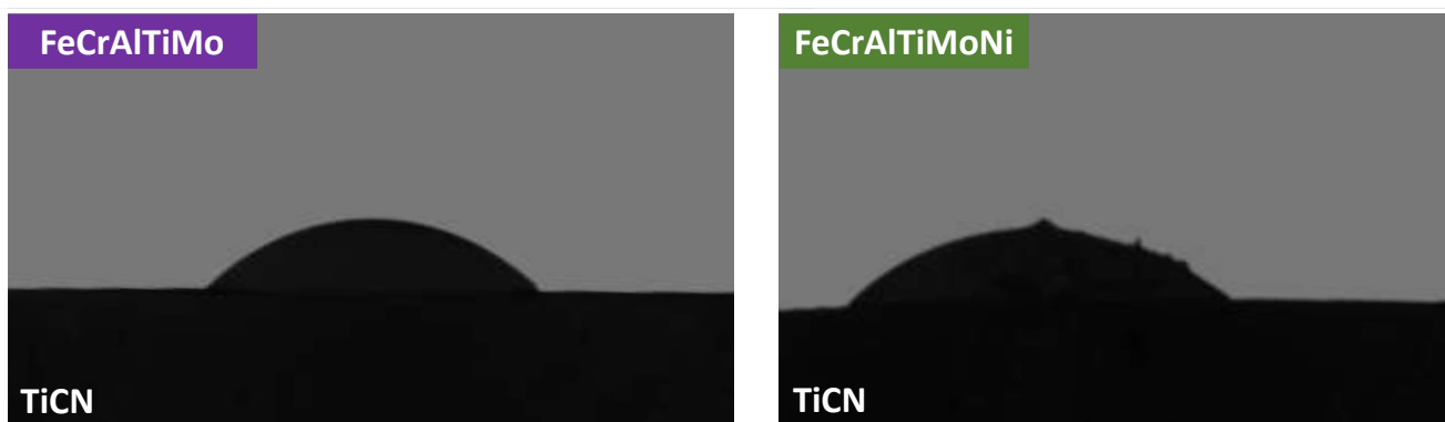
Figure 5. High temperature wetting experiments of FeCrAlTiMo (HEA-5) on a TiCN substrate and FeCrAlTiMoNi (HEA-6) on a TiCN substrate.
